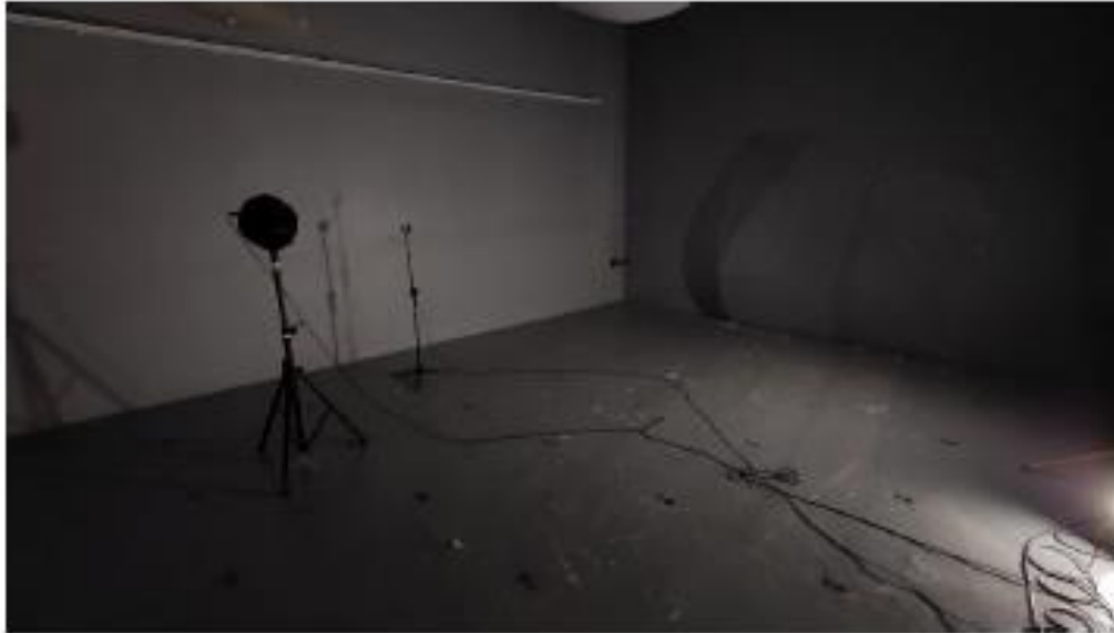
Figure 1: reverberation chamber assembly with source only
